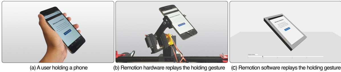
Fig. 1. The concept of Remotion: the system can capture and replay the mobile device interactions in remote usability testing. For example, if (a) a user is holding a phone, the Remotion system can record data for this moment and replay using (c) software and (b) hardware visualizations.
